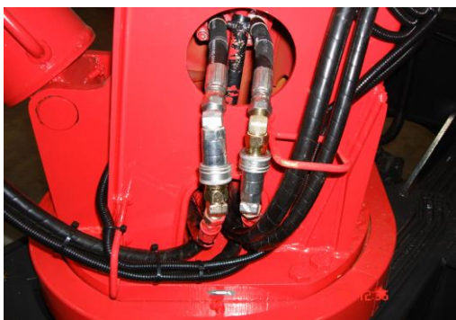
Illustration 5 showing crane ready for emergency winching
