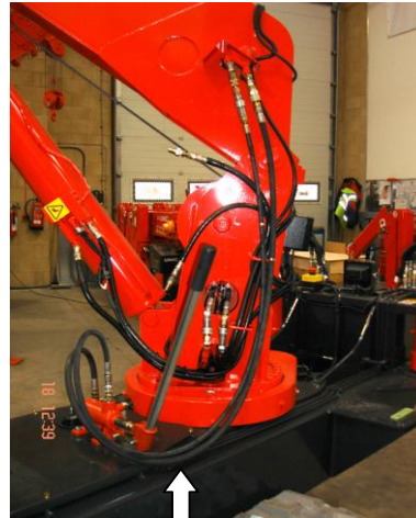
Illustration 3 showing crane ready for emergency telescoping. Note the telescoping adaptor (D) fitted to the line
